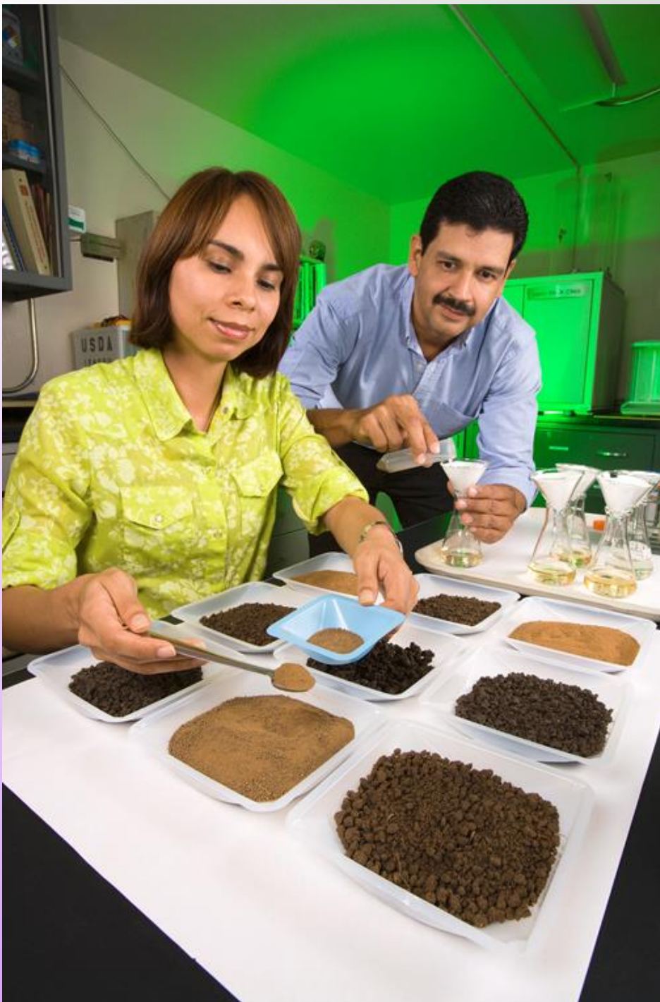
Technicians process soil samples for organic matter analysis. (courtesy USDA)
