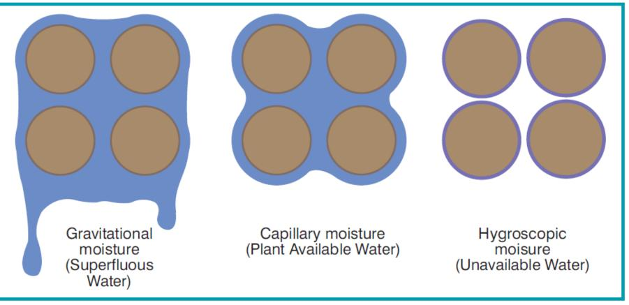
FIGURE 2. Three types of moisture found in soils.
