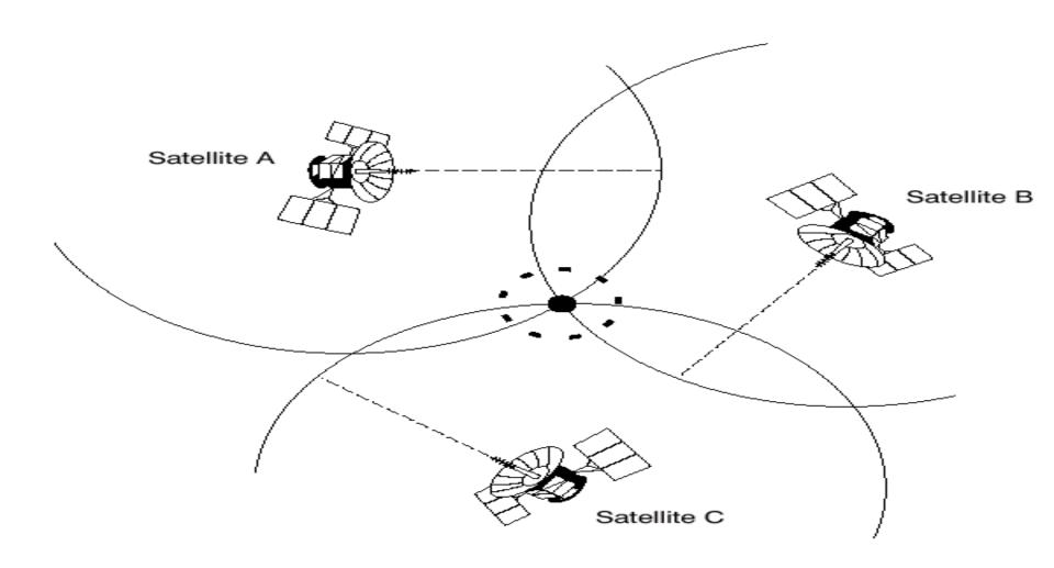
Positions on the earth are determined by measuring the distance from a group of satellites in space.
